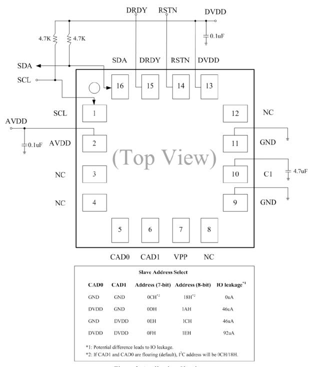
Figure 2. Application Circuit
