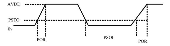
PSTO: Power Supply Turn Off voltage PSOI: Power Supply Turn Off Interval
